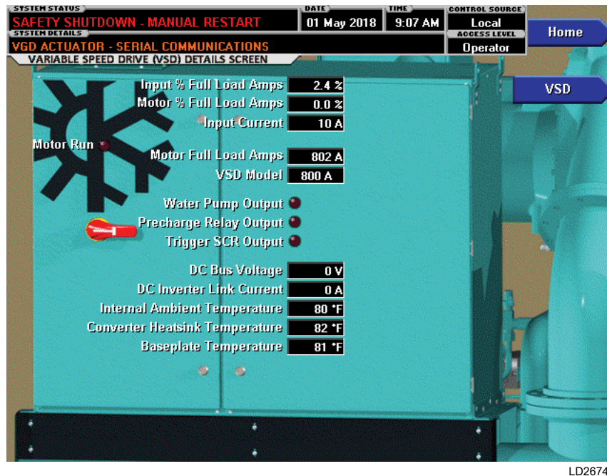
FIGURE 19 - VARIABLE SPEED DRIVE (VSD) DETAILS SCREEN
