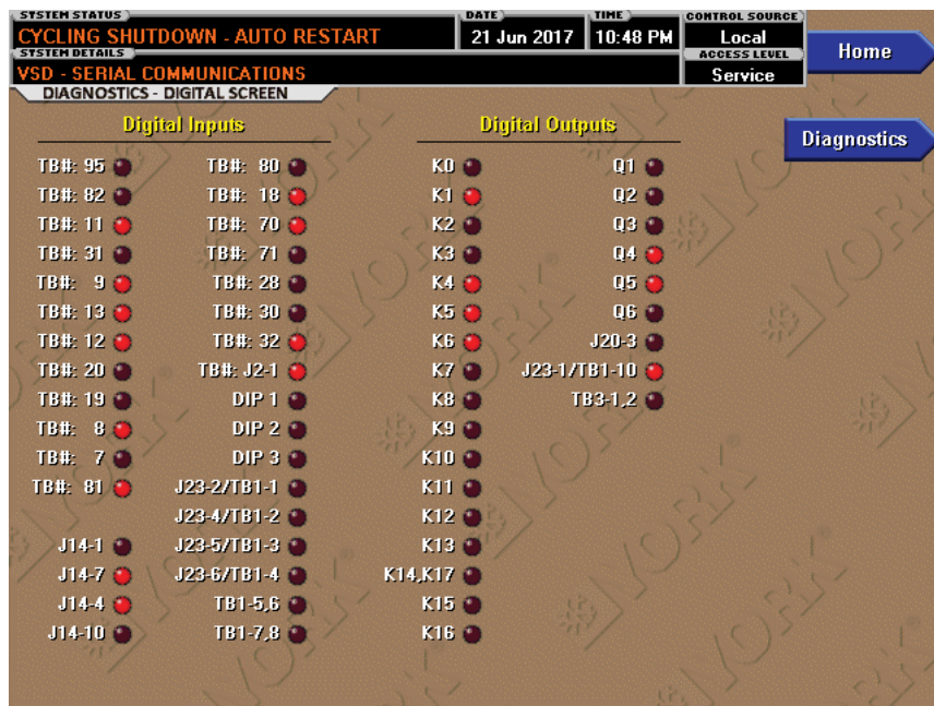
FIGURE 102 - DIGITAL INPUTS / OUTPUTS TEST SCREEN
