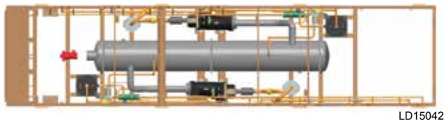
FIGURE 10 - 2-PASS EVAPORATOR OPTIONAL ARRANGEMENT
