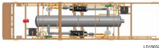
FIGURE 9 - 2-PASS EVAPORATOR STANDARD ARRANGEMENT
