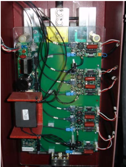
FIG. 11 – SCR POWER STACK ASSEMBLIES
