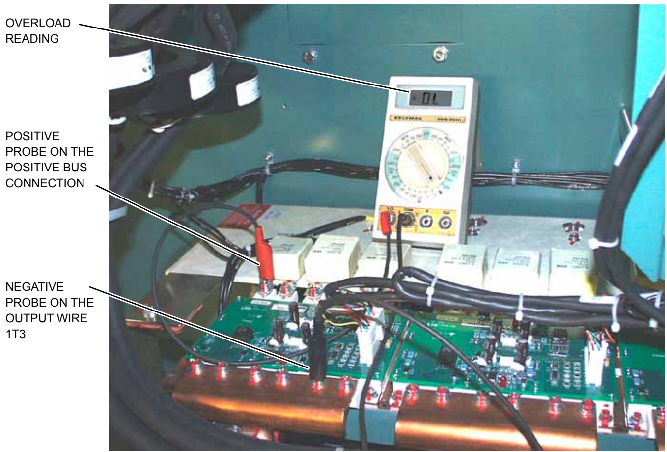
FIGURE 26 - 385/419/503/608 HP DRIVE IGBT MODULE VERIFICATION #1
