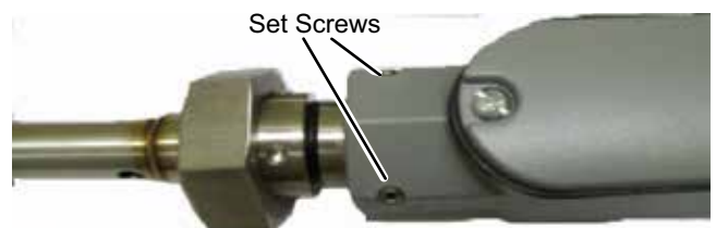
FIGURE 12 - CS02 SENSOR PROBE MOUNTING
