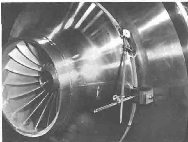
DETAIL A - CHECKING RIM RUN-OUT TOLERANCE: MODELS 108, 120 & 126 = .005" MODELS 131 & 144 = .006"
