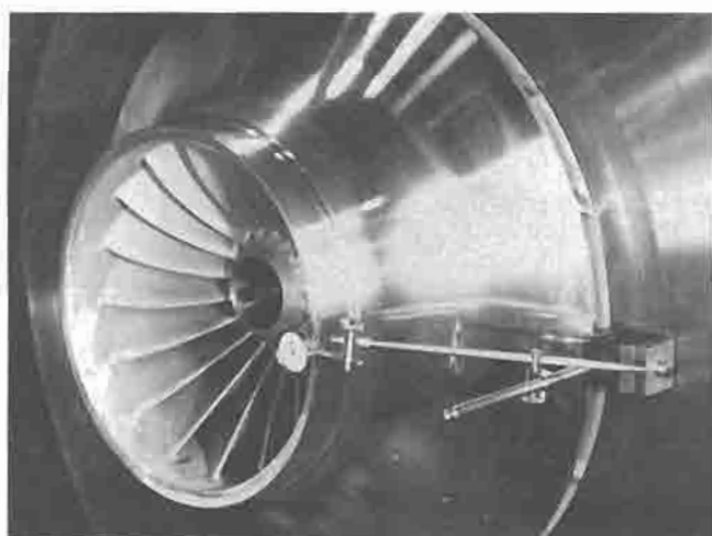
DETAIL C - CHECKING AXIAL THRUST TOLERANCE = .007" TO .014"
