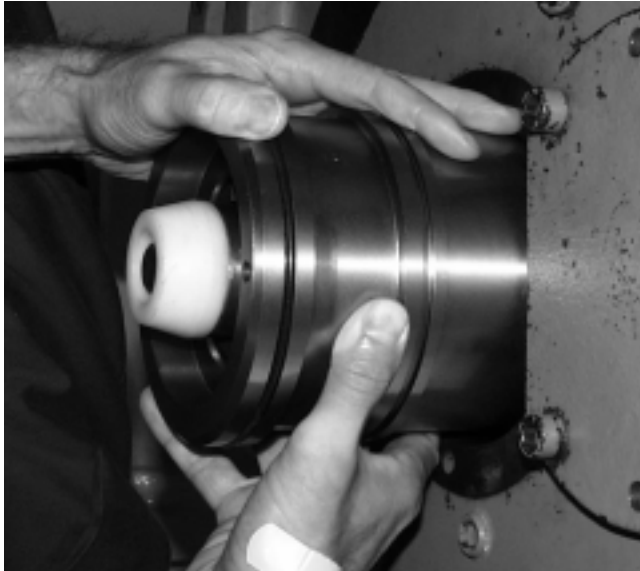
FIG. 14 – SEAL HOUSING SPACER INSTALLATION
