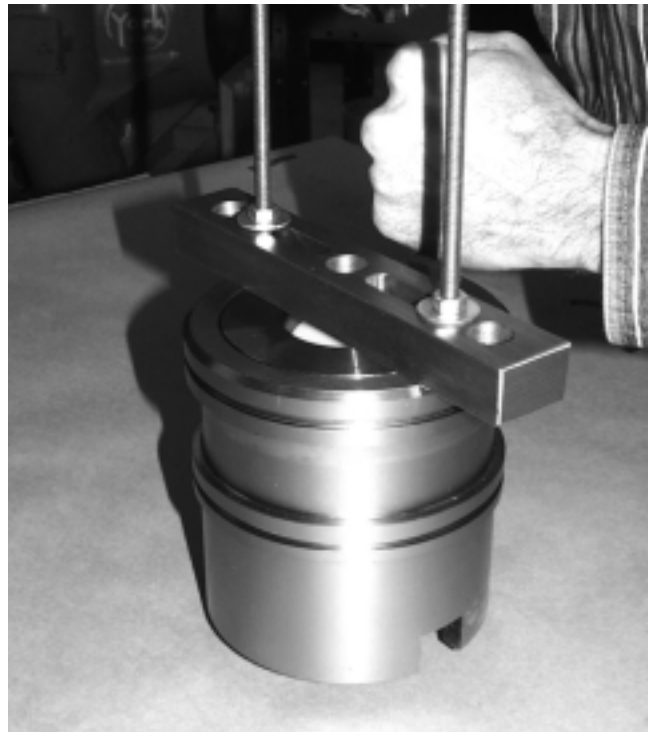
FIG. 13 – PUTTING SEAL HOUSING SPACER ONTO INSTALLATION TOOL
