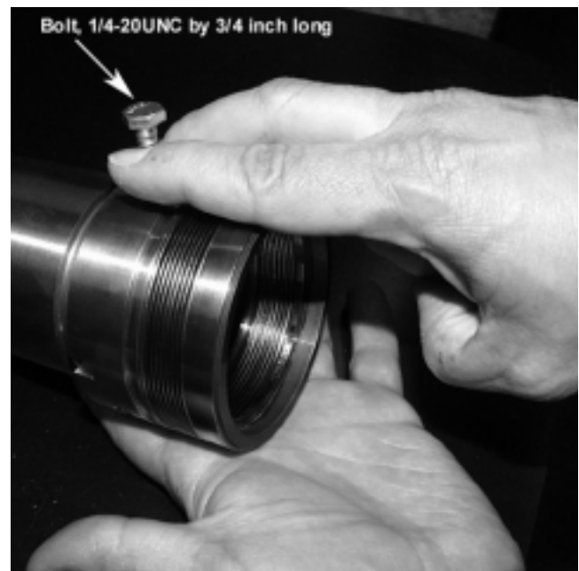
FIG. 3 – INSTALLING BOLT FOR SEAL REMOVAL
