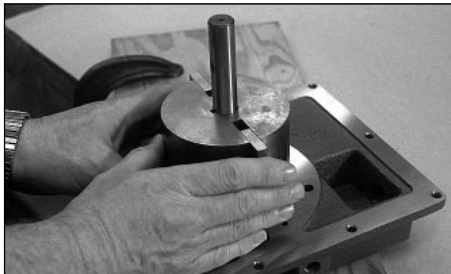
Figure 3 - Sliding Vanes out of Rotor Slot
