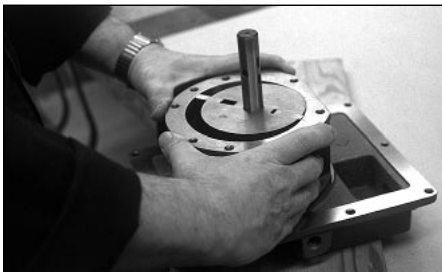
Figure 5 - Centering the Seal Machined in the Stator Bore on the Rotor
