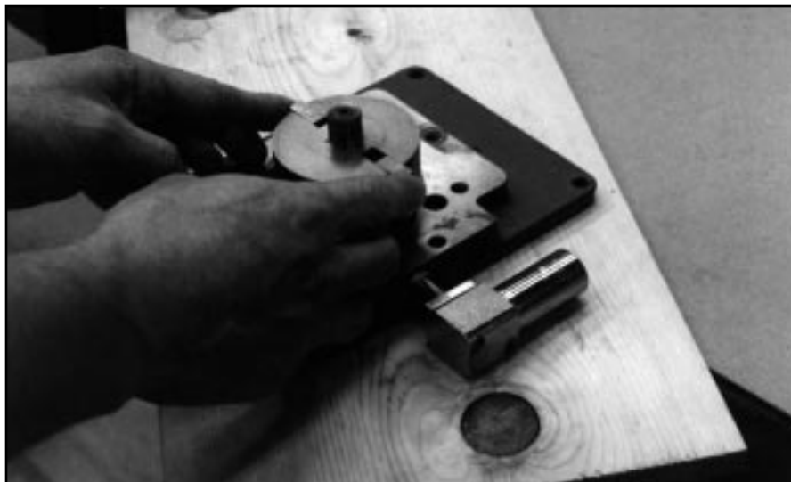
Figure 3 - Inserting the Vanes in the Rotor Slot
