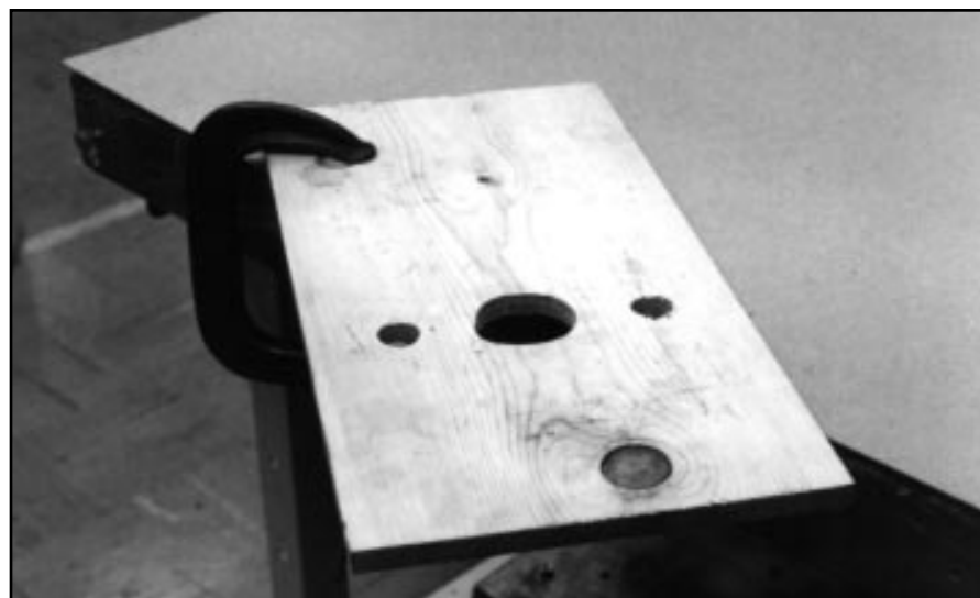
Figure 1 - A simple assembly fixture
