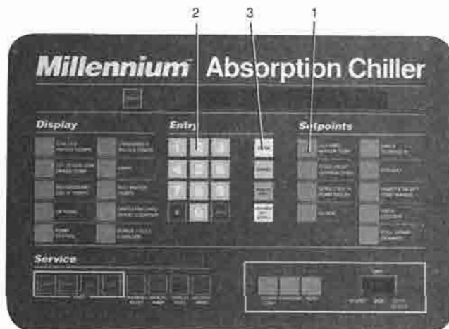
FIG. 5 - KEYPAD - PROGRAMMING "LEAVING HOT WATER TEMP" SETPOINT
