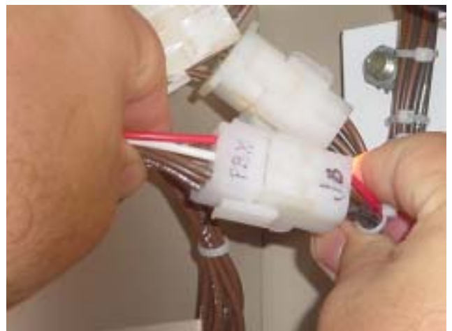
FIG. 12 - CONNECTING SMART RELAY HARNESS
