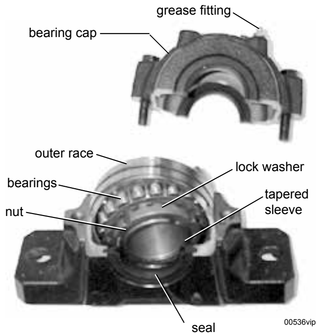
FIGURE 30 - SPLIT BEARING
