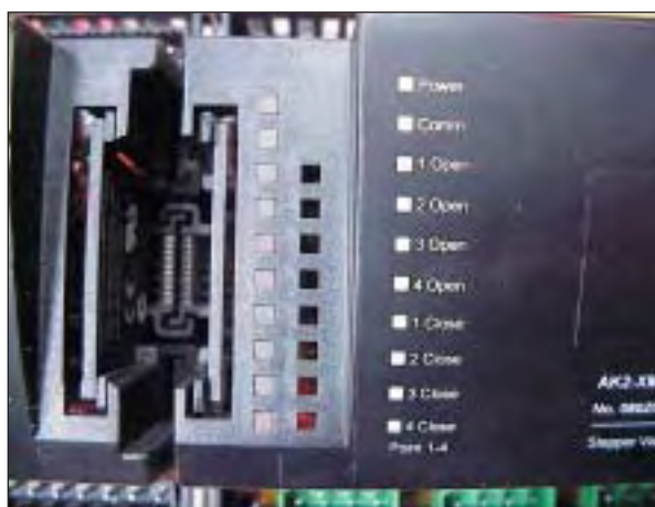
FIG. 41 -POWER, COMMS AND SYSTEM OPEN/ CLOSE LED'S
