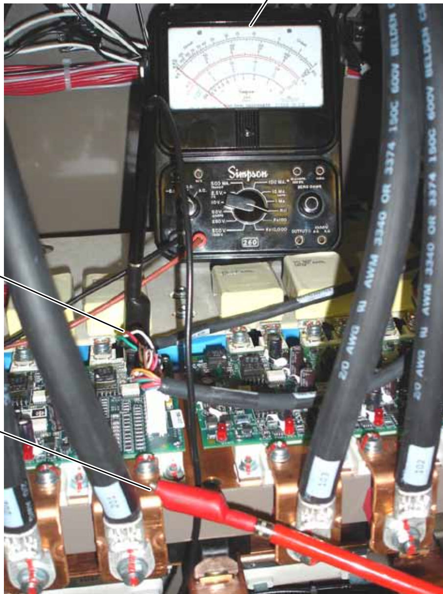
FIGURE 8 - IGBT MODULE VERIFICATION (REFERENCE STEP 7)
