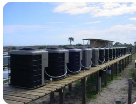
Graph 3 , Left: Tianjin, China (identified as city with top 10 worst air pollution). Right: New Smyrna Beach, FL (Severe subtropical marine environment, category C4/C5 corrosive environment (ISO 9223))
