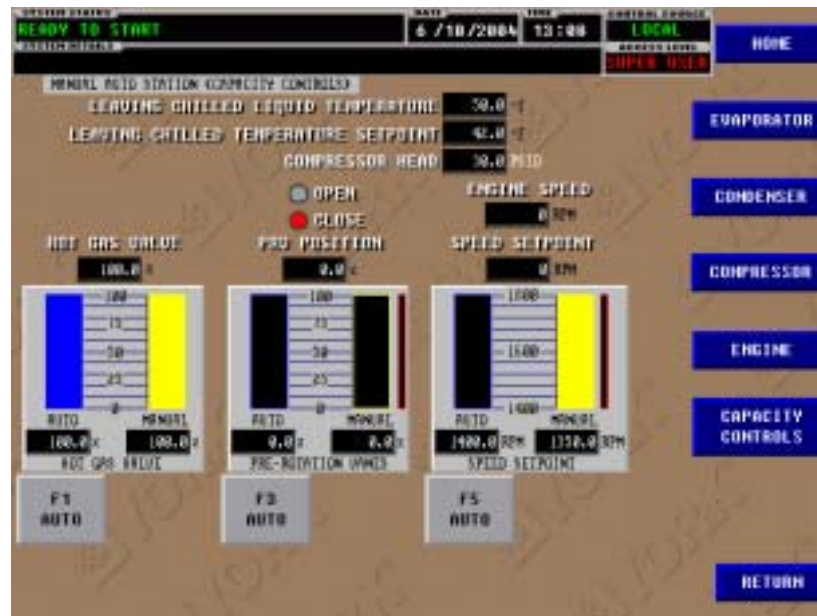
FIG. 18 - MANUAL/AUTO STATION (CAPACITY CONTROLS) SCREEN
