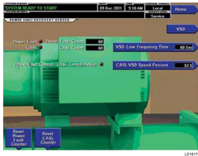
FIGURE 120 - POWER FAULT RECOVERY SCREEN
