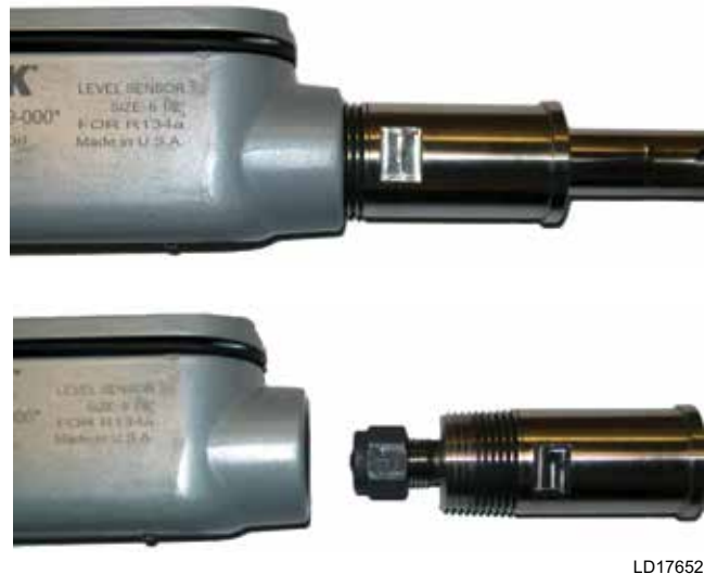
FIGURE 7 - CS01 ELECTRICAL ENCLOSURE THREADED ONTO PROBE ASSEMBLY
