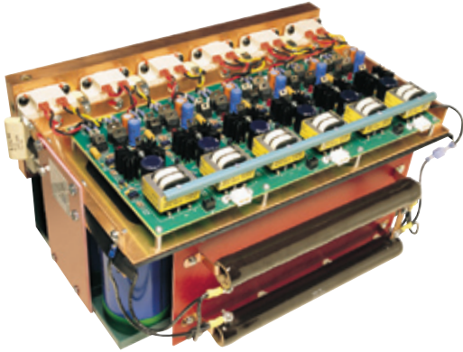
The pole assemblies of the OptiSpeed drive start the chiller motor gently.
