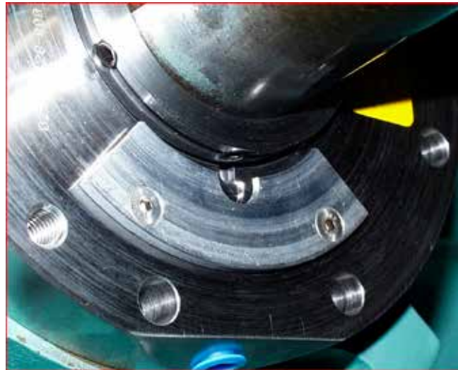
FIGURE 11 - RETAINER RUNNING POSITION LD22342
