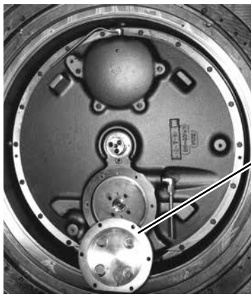
FIGURE 24 - LOW-SPEED THRUST BEARING REMOVED
