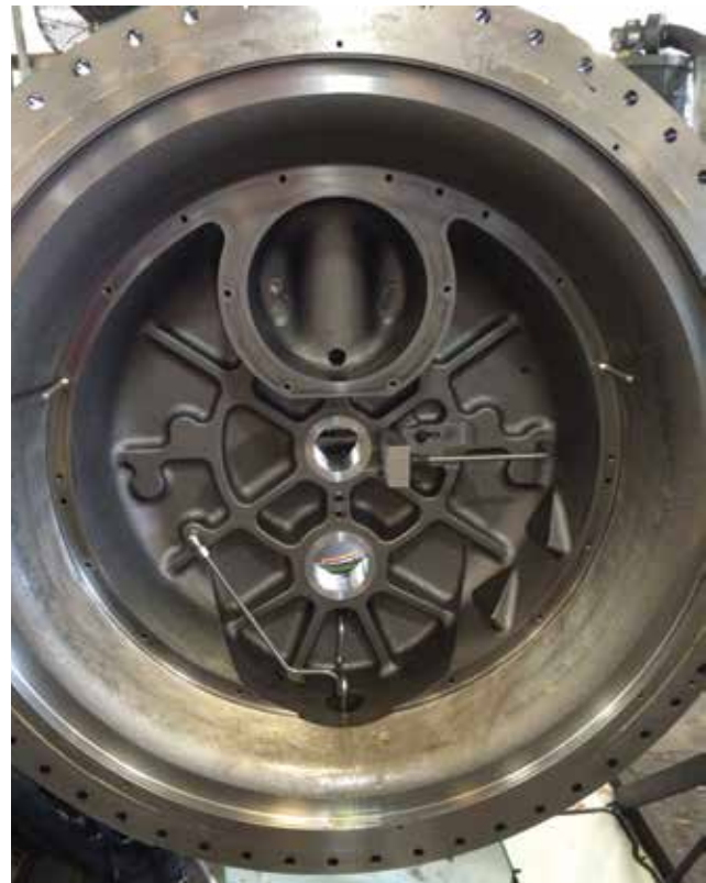
FIGURE 32 - BEARING HOUSING REMOVED
