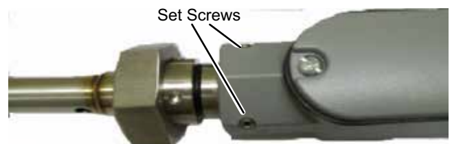
FIGURE 12 - CS02 SENSOR PROBE MOUNTING
