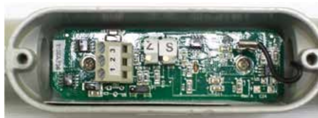
FIGURE 9 - HANSEN SIGNAL TRANSMITTER BOARD – WITH AND WITHOUT POTTING COMPOUND
