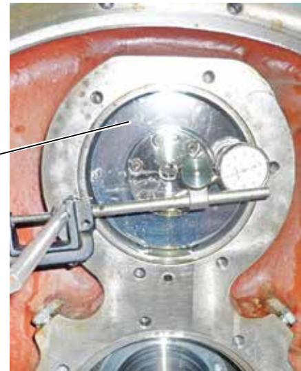
FIGURE 40 - CHECKING HIGH-SPEED THRUST COLLAR RUN-OUT
