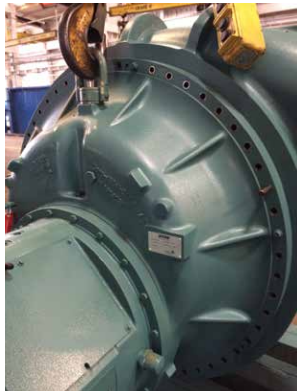
FIGURE 13 - DISASSEMBLY OF ROTOR SUPPORT FROM THE ROTOR SCROLL
