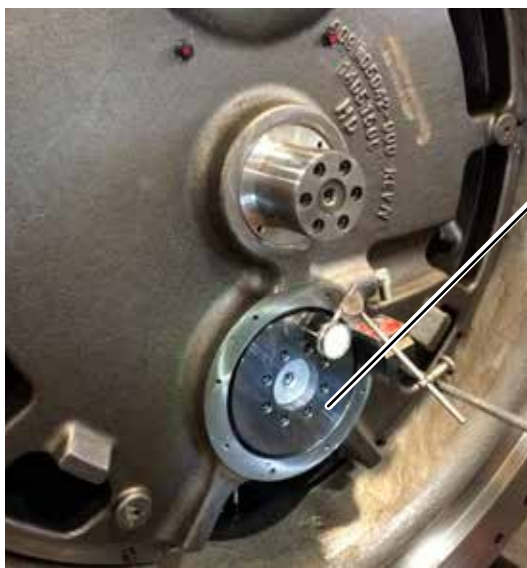
FIGURE 25 - CHECKING LOW-SPEED THRUST RUNOUT
