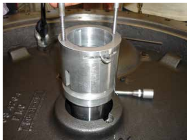
FIGURE 29 - FRONT HIGH-SPEED BEARING REMOVAL
