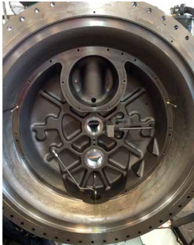
FIGURE 32 - BEARING HOUSING REMOVED
