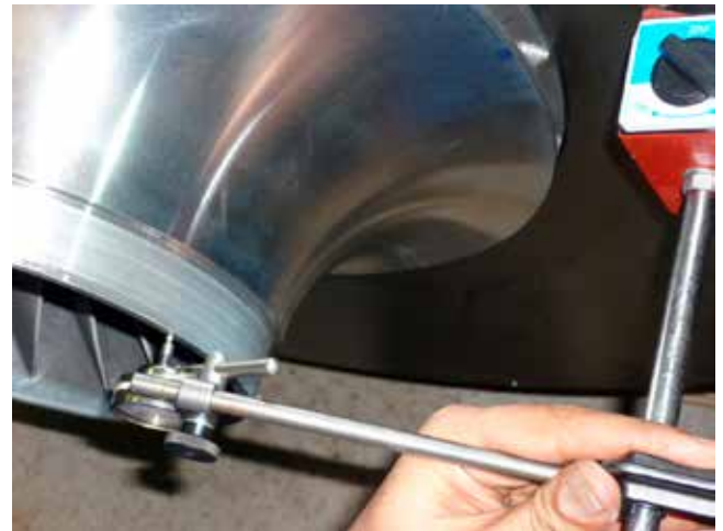
FIGURE 16 - DETAIL C – CHECKING AXIAL THRUST
