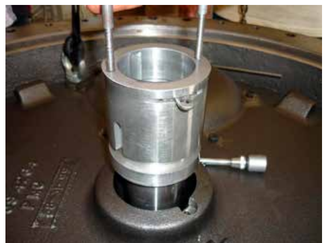
FIGURE 29 - FRONT HIGH-SPEED BEARING REMOVAL
