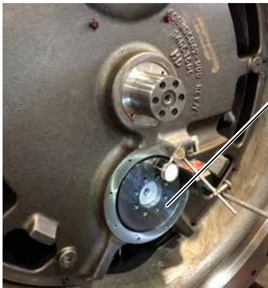
FIGURE 25 - CHECKING LOW-SPEED THRUST RUNOUT
