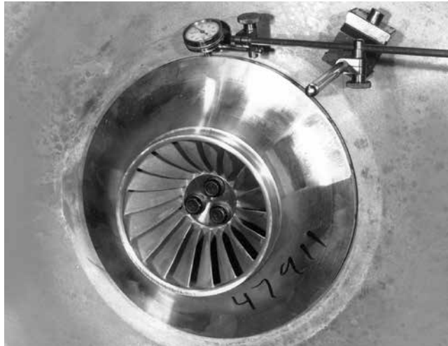
FIGURE 14 - DETAIL A – CHECKING RIM RUNOUT
