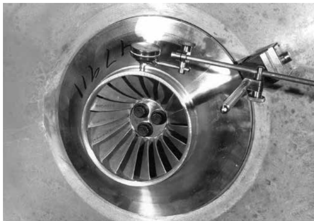
FIGURE 15 - DETAIL B – CHECKING EYE RUNOUT
