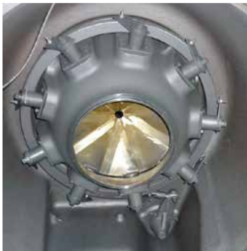
FIGURE 62 - PRE-ROTATION VANE HOUSING ASSEMBLY
