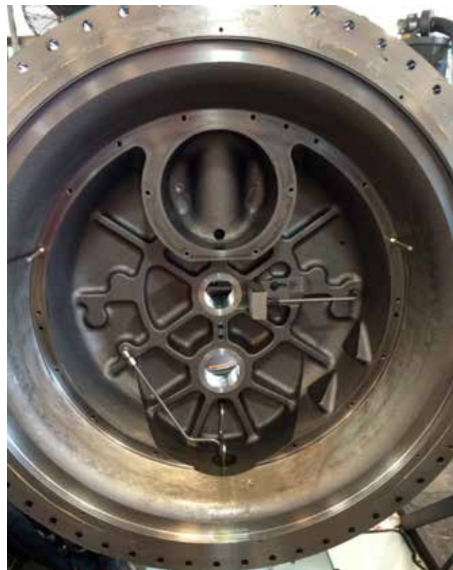
FIGURE 32 - BEARING HOUSING REMOVED
