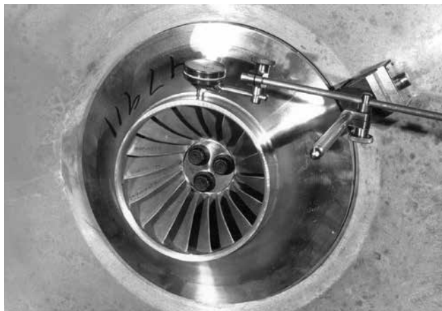
FIGURE 15 - DETAIL B – CHECKING EYE RUNOUT
