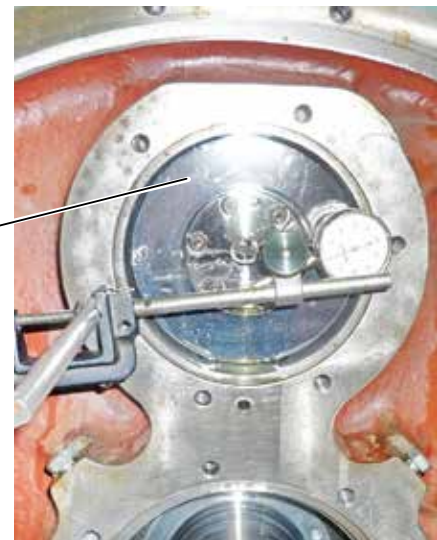
FIGURE 40 - CHECKING HIGH-SPEED THRUST COLLAR RUN-OUT
