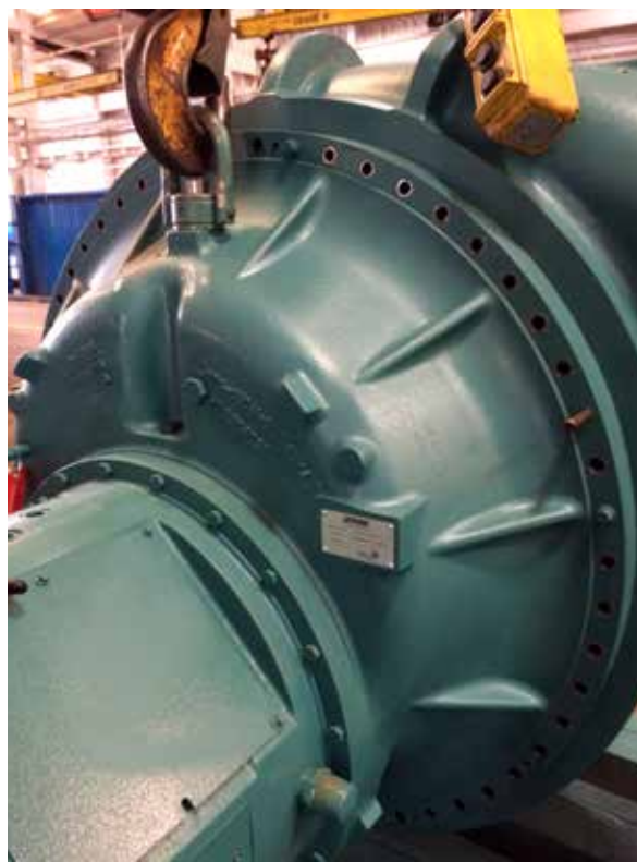
FIGURE 13 - DISASSEMBLY OF ROTOR SUPPORT FROM THE ROTOR SCROLL
