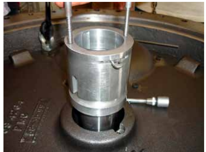
FIGURE 29 - FRONT HIGH-SPEED BEARING REMOVAL
