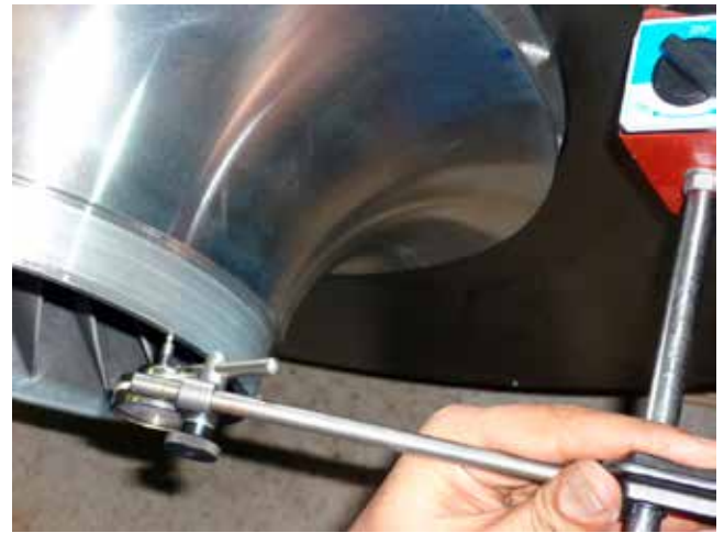
FIGURE 16 - DETAIL C – CHECKING AXIAL THRUST
