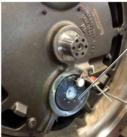
FIGURE 25 - CHECKING LOW-SPEED THRUST RUNOUT
