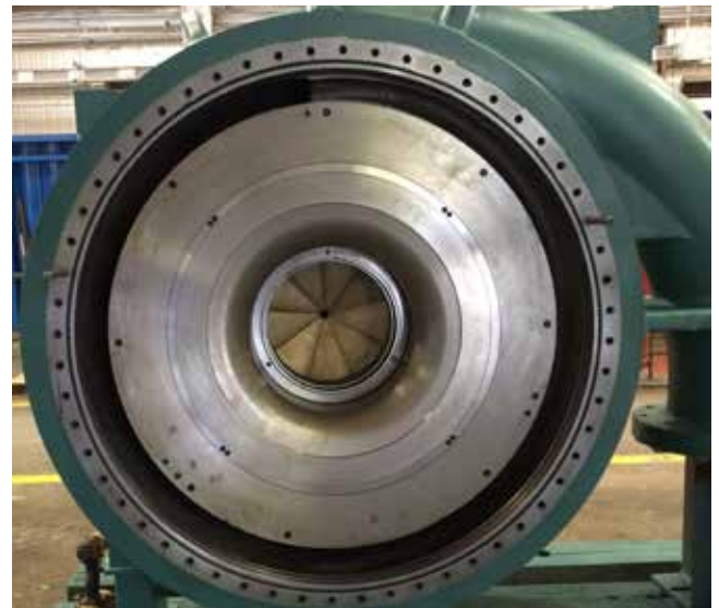
FIGURE 59 - SCROLL HOUSING READY FOR RE-ASSEMBLY TO MOTOR SUPPORT
