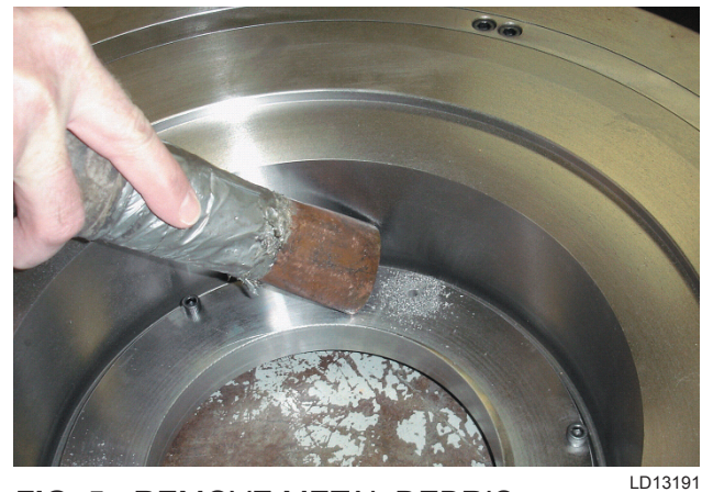
FIG. 5 - REMOVE METAL DEBRIS
