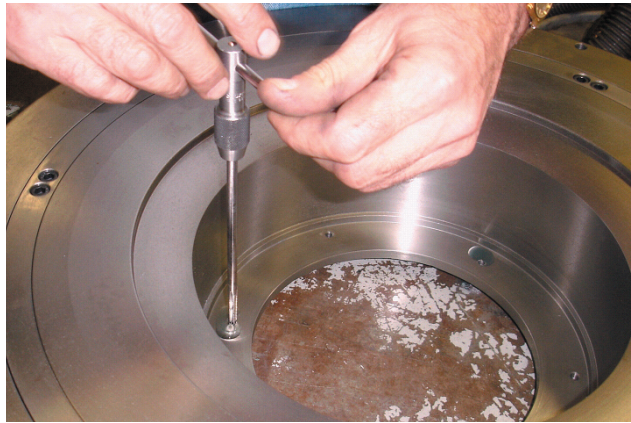
FIG. 6 - TAP THE DRILLED HOLES
