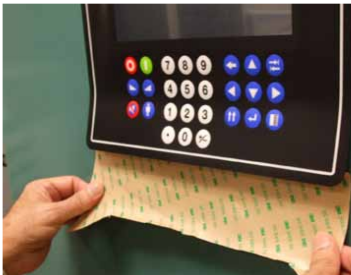
FIGURE 9 - PULL PAPER BACKING OFF KEYPAD/TOUCH-SCREEN
