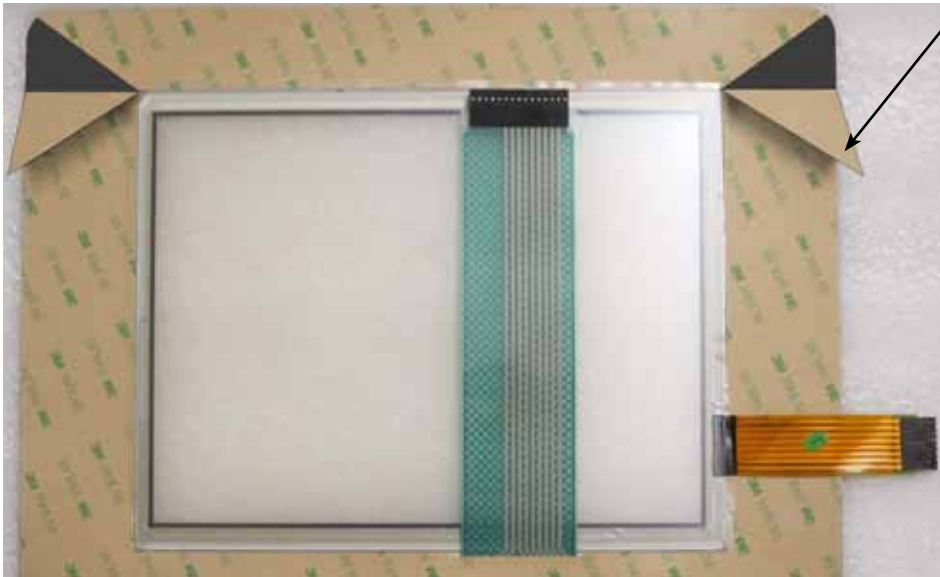
FIGURE 6 - CUTTING ADHESIVE PAPER BACKING
