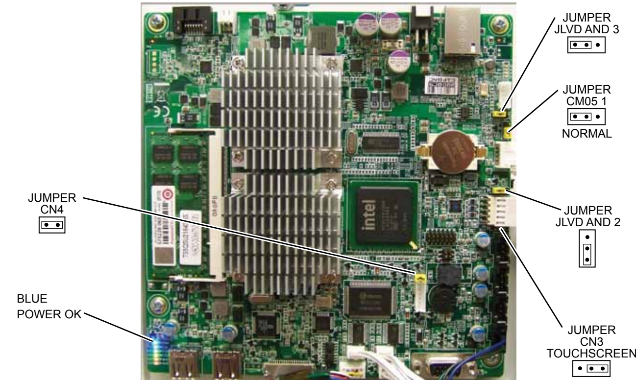
FIGURE 2 - QUANTUM™ LX JUMPER SETTINGS
