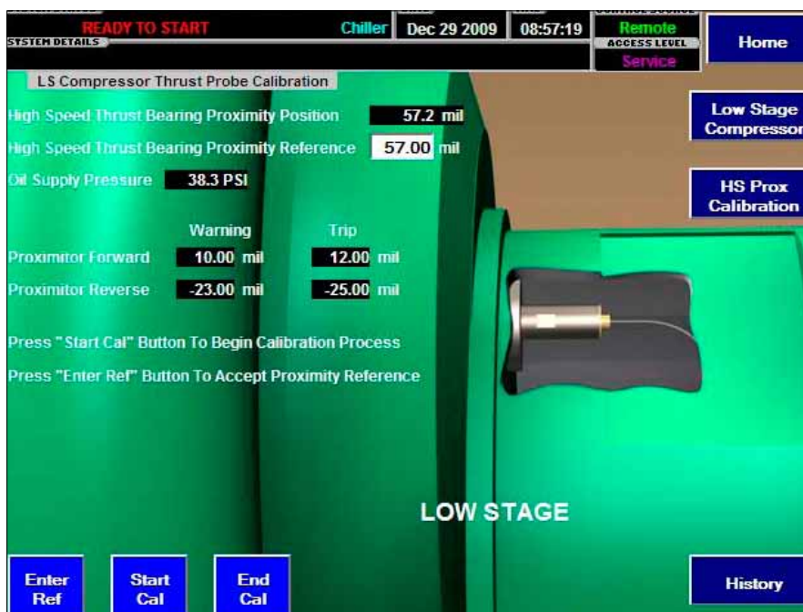
FIGURE 46 - HS PROXIMITY CALIBRATION SCREEN
