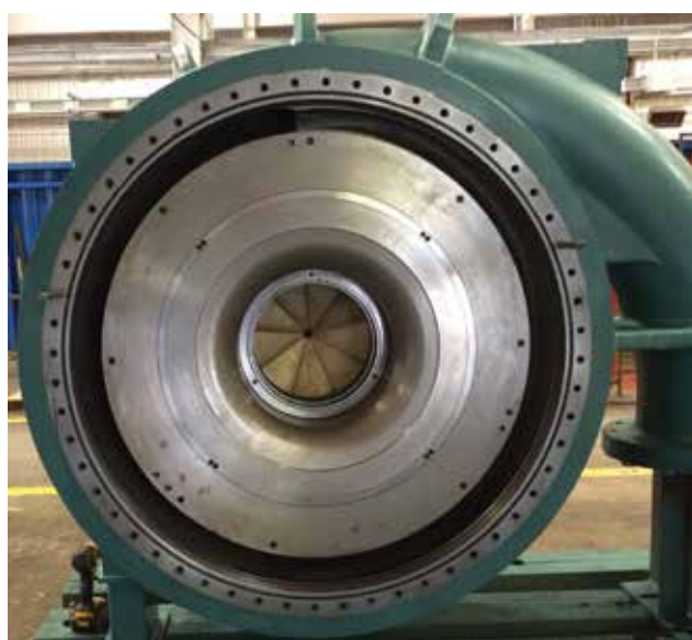
FIGURE 59 - SCROLL HOUSING READY FOR RE-ASSEMBLY TO MOTOR SUPPORT
