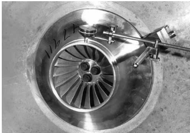
FIGURE 15 - DETAIL B – CHECKING EYE RUNOUT
