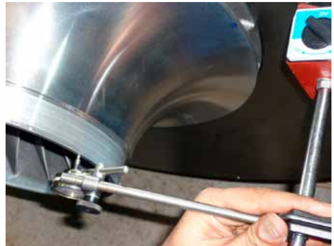
FIGURE 16 - DETAIL C – CHECKING AXIAL THRUST
