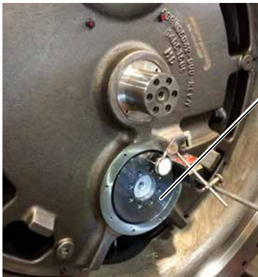
FIGURE 25 - CHECKING LOW-SPEED THRUST RUNOUT
