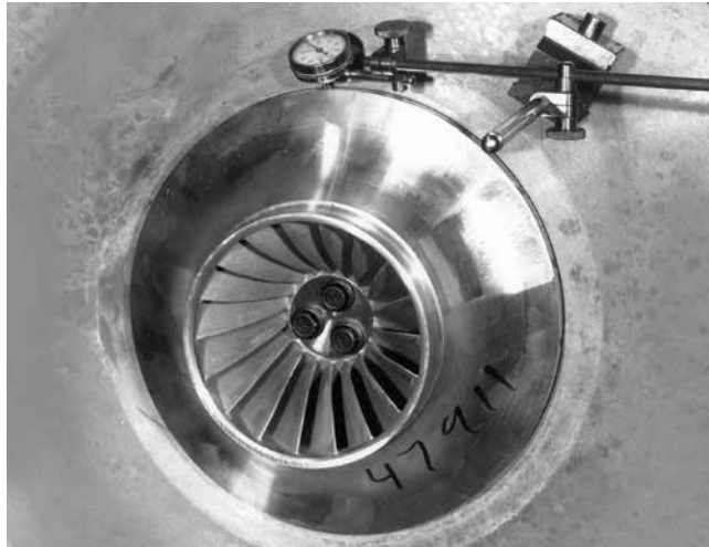
FIGURE 14 - DETAIL A – CHECKING RIM RUNOUT
