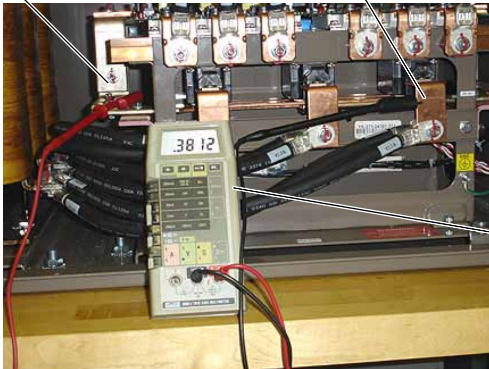
FIGURE 15 - SCR / DIODE MODULE VERIFICATION (REFERENCE STEP 11)
