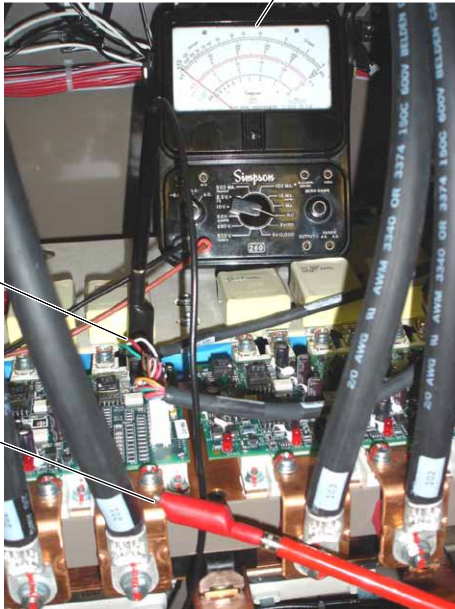
FIGURE 8 - IGBT MODULE VERIFICATION (REFERENCE STEP 7)
