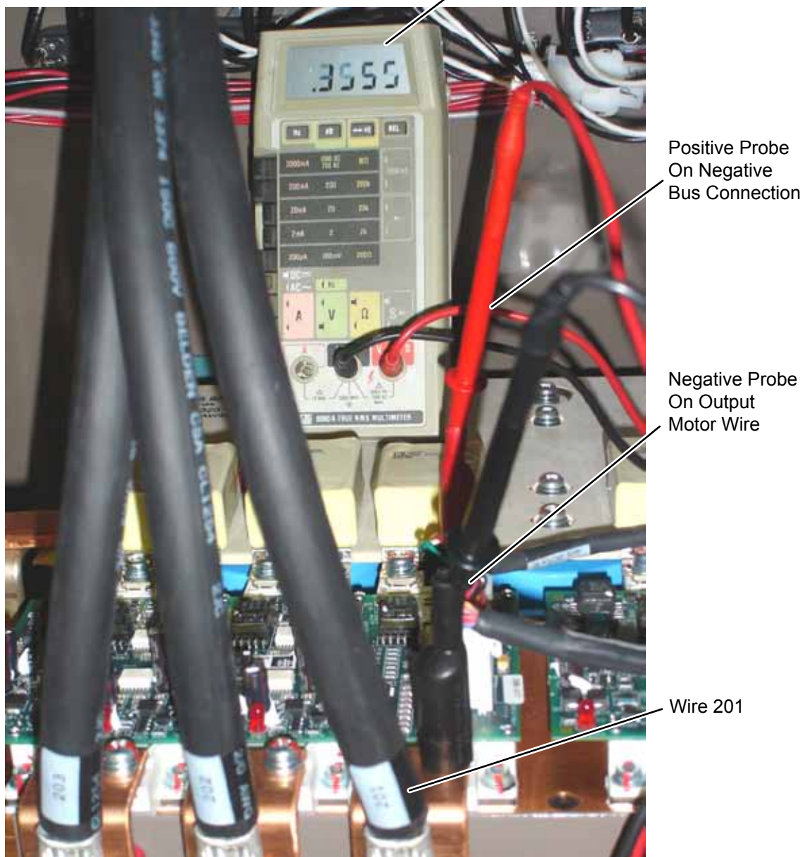
FIGURE 7 - IGBT MODULE VERIFICATION (REFERENCE STEP 1)
