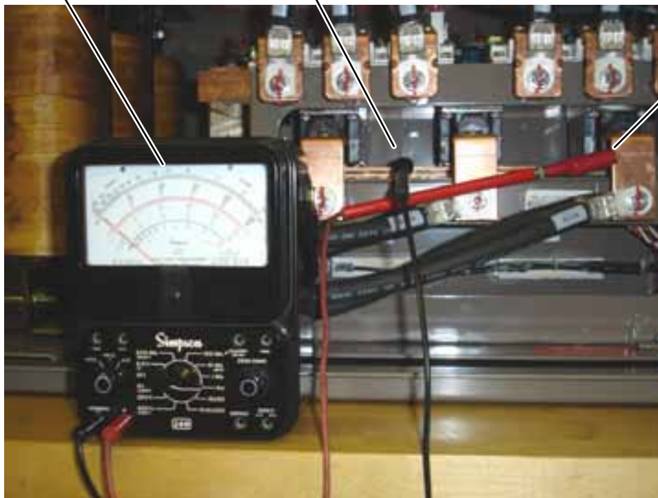
FIGURE 11 - SCR / DIODE MODULE VERIFICATION (REFERENCE STEP 1)
