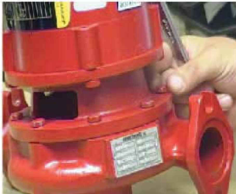
FIGURE 3 - LOOSENING THE BOLTS ATTACHING THE IMPELLER ADAPTER TO THE VOLUTE HOUSING
