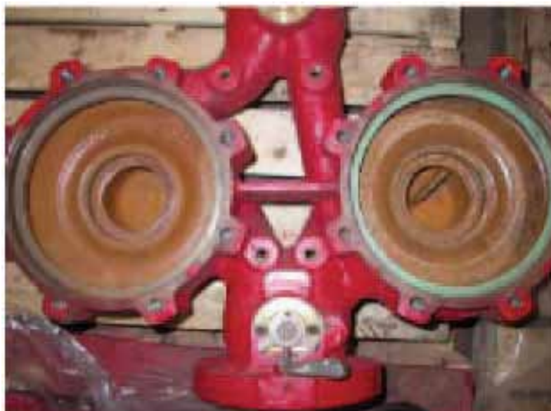
FIGURE 1 - CORRODED WATER PUMP VOLUTES
