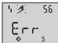
Example Error caused by pin position
