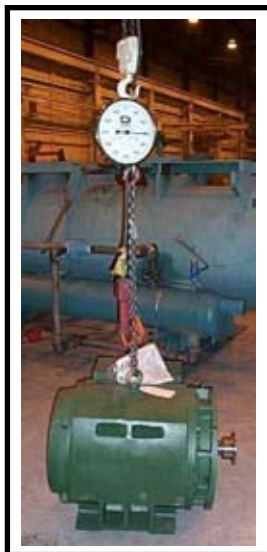
Figure 14. Weigh replacement motor
