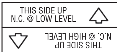
Nameplate Position for Low Level Alarm
