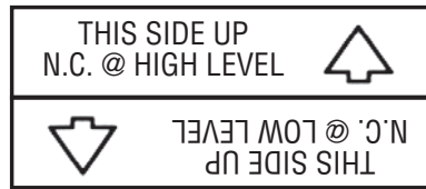
Nameplate Position for High Level Alarm
