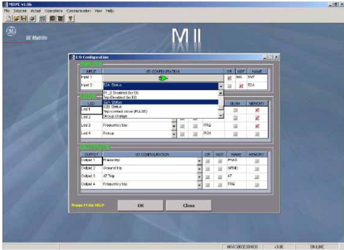
Figure 6-3: SIMPLE ACTION INPUT CONFIGURATION (ONE ELEMENT ASSIGNMENT)
