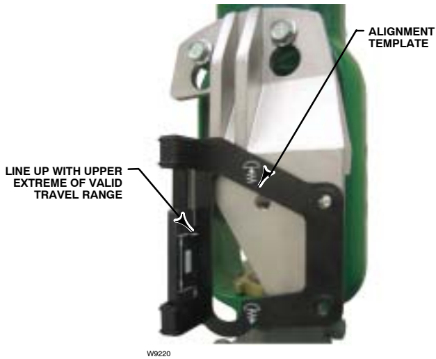
Figure 2-4. Air-to-Open Magnet Array Alignment
