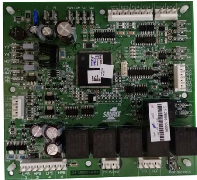
FIGURE 9 : Four-Stage Controller SE-SPU1004-0 (031-03032-000A / 1034521)
