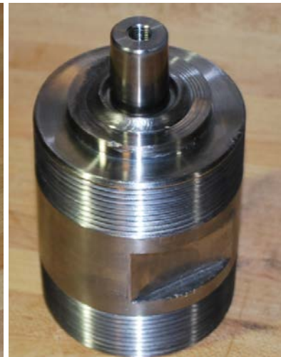
(Fig 14 Machined test coupon with Pop-A-Plug)
