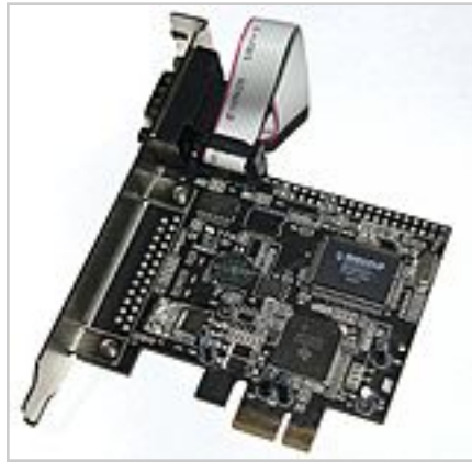
PCI Express x1 card with one RS-232 port
