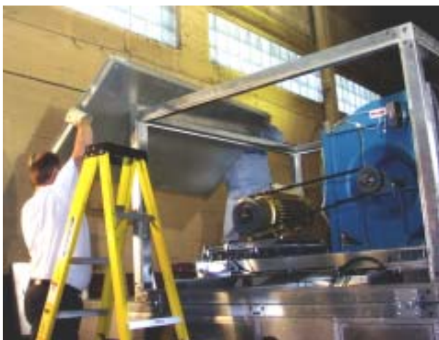
FIG. 6 - REMOVE TOP PANELS
