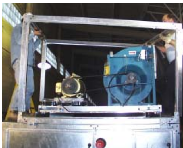
FIG. 7 - REMOVE TOP RACEWAY ASSEMBLY
