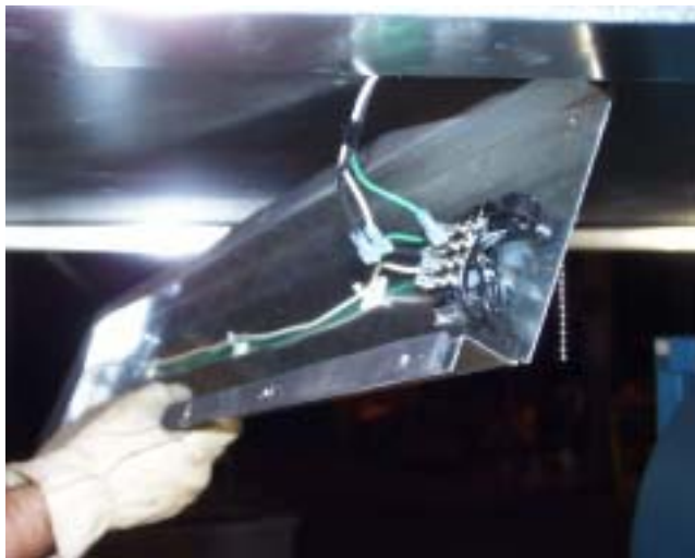
FIG. 16 - REMOVE ELECTRICAL CONNECTORS
