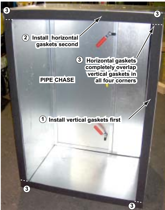
FIG. 2 – APPLY GASKET TO PIPE CHASE
