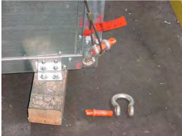
FIG. 1-4 – PROPER LIFTING WITH SHACKLE AT CORNER
