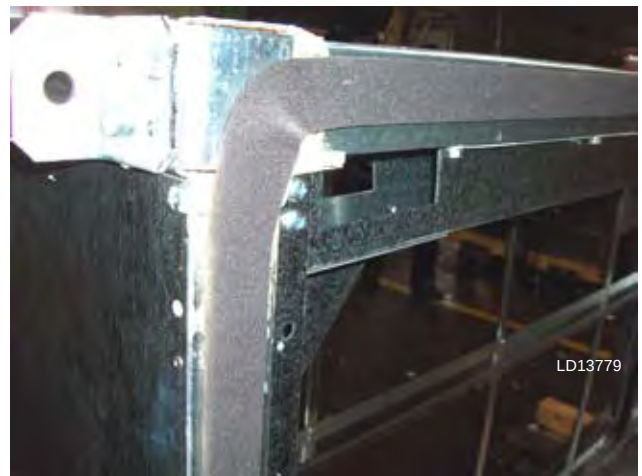
FIG. 2-21 – APPLYING GASKET TO SHIPPING SPLIT
