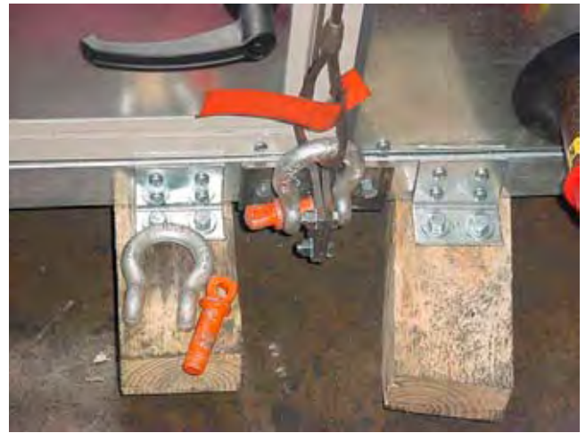
FIG. 1-5 – PROPER LIFTING WITH SHACKLE AT LIFTING LUG
