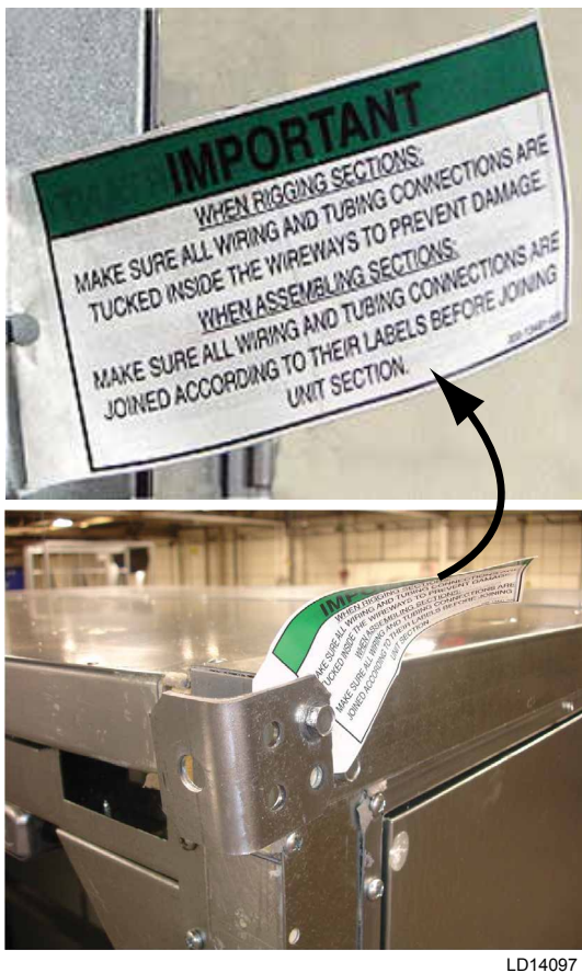
FIGURE 60 - REMOVE AND REPOSITION SHIPPING SPLIT ANGLE
