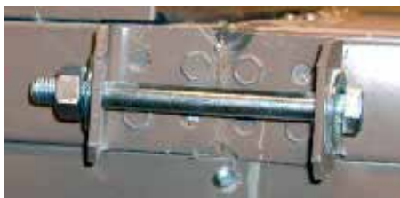
Raceway Lifting Lugs Assembled
