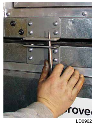
FIGURE 68 - GUIDE BRACKETS TOGETHER
