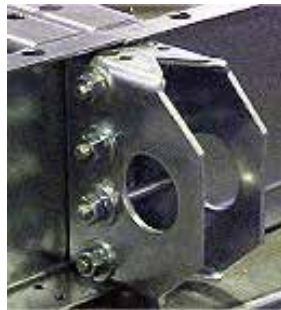
Baserail Lifting Lugs Assembled
