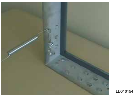
FIGURE 42 - CORRECT LATCH/KNOCKOUT CONFIGURATION
