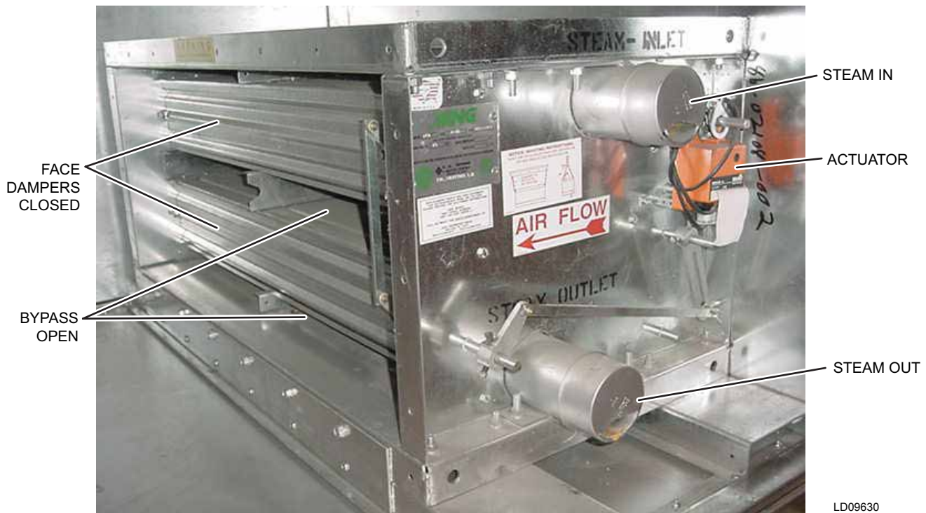
FIGURE 31 - INTEGRAL FACE AND BYPASS COIL (HORIZONTAL TUBES, STEAM SHOWN)
