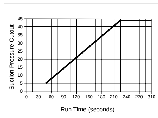
Suction Pressure Cutout With 44 PSIG Programmed Cutout
