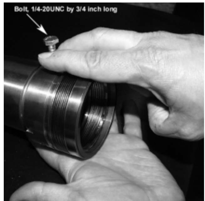
FIG. 3 – INSTALLING BOLT FOR SEAL REMOVAL
