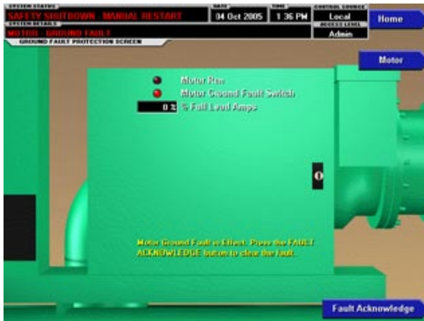
FIG. 15A- GROUND FAULT PROTECTION SCREEN
