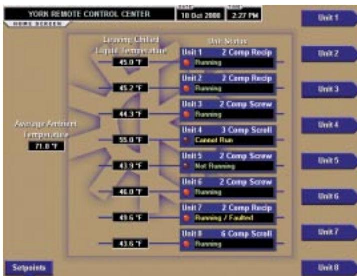
View the status of up to eight chillers on the OptiView Panel's Home Screen
