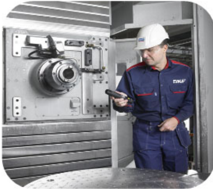
Figure 10 – 30. Monitor the Speed with a Tachometer.
