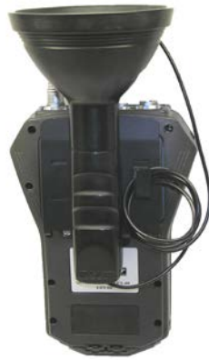
Figure 11 - 8. The Microphone/Parabolic Reflector Connected to the Microlog.
