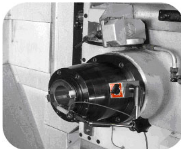
Figure 10 – 13. Perform a Nose Run-Out Test.
