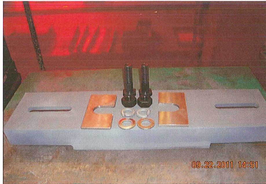
Fabricate top portion of bracket. 1/4" block to be used during this operation, shim packs to be installed during step 10.
