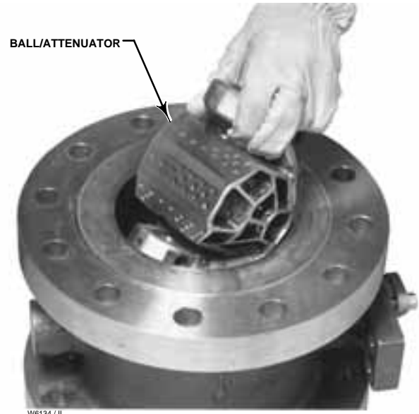
Figure 18. Ball/Attenuator Installation and Removal Method
